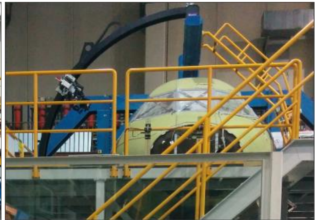
Figure 13. Different views of the Mechanical Subsystem (supporting the NDT System) integrated with the test rig at Topic Manager facilities
