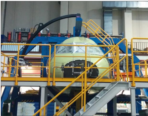
Figure 13. Different views of the Mechanical Subsystem (supporting the NDT System) integrated with the test rig at Topic Manager facilities
