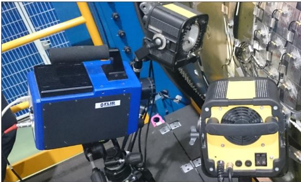
Figure 4: Hedler H25s halogen lamps that forms the Excitation Subsystem
