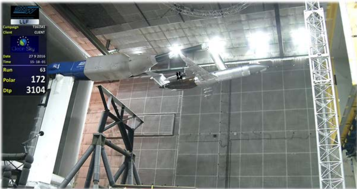
Figurer 4: Z08 model in DNW-LLF open test section during acoustic test phase
