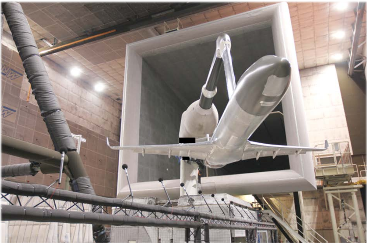
Figure 2: Z08 model in DNW-LLF open test section during commissioning phase, wind-off
