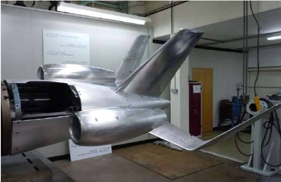
Empennage / Nacelle Asm (with alternative central VTP attached solely to confirm interfacing)
