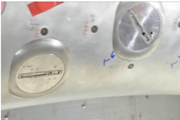
Figure 2 - Multiple Degree of Freedom CTA Probe Traverse Mechanisms & Fairings
