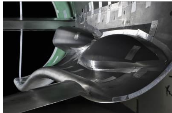
Figure 2 - Multiple Degree of Freedom CTA Probe Traverse Mechanisms & Fairings
