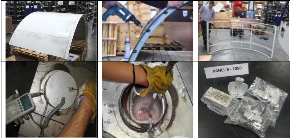
Figure 3. Live dismantling (upper line) of panels and live remelting of sorted aluminium alloys (bottom line)
