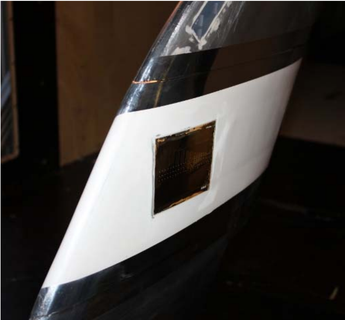
figure 28: model equipped with surface sensors
