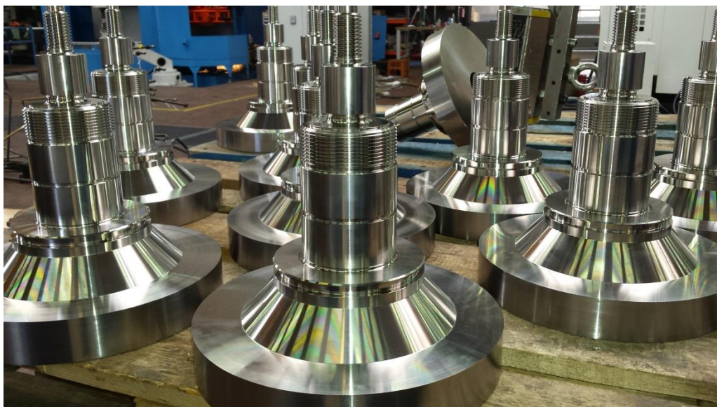
Figure 5: Cranks following initial turning before milling @ Germany machining plant
