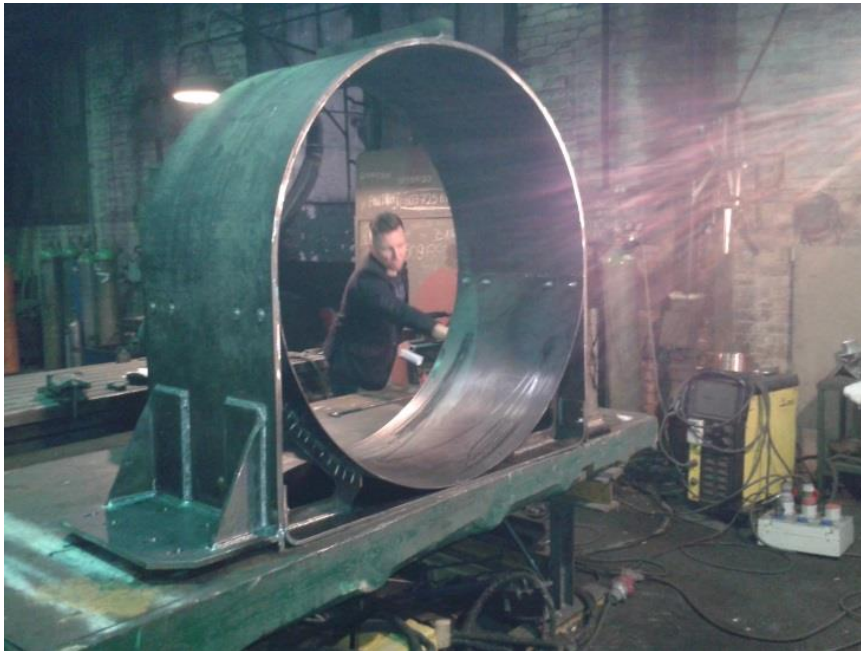
Figure 6: Containment Case undergoing inspection following welding @ Poland welding plant
