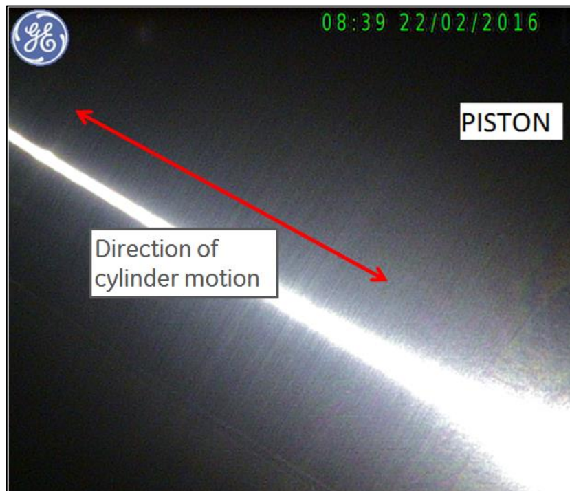
Figure 3: Piston surface following test campaign
