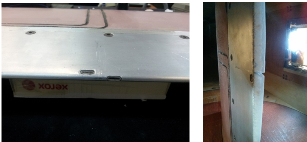
Figure 1: The sensor setup(left) and the test bed aerofoil mounted in the ice tunnel (right).
