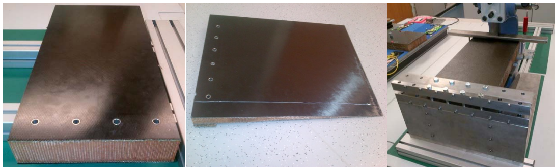
Figure 6: Photos of the coupon, subcomponent and the fixation with the mounted coupon
