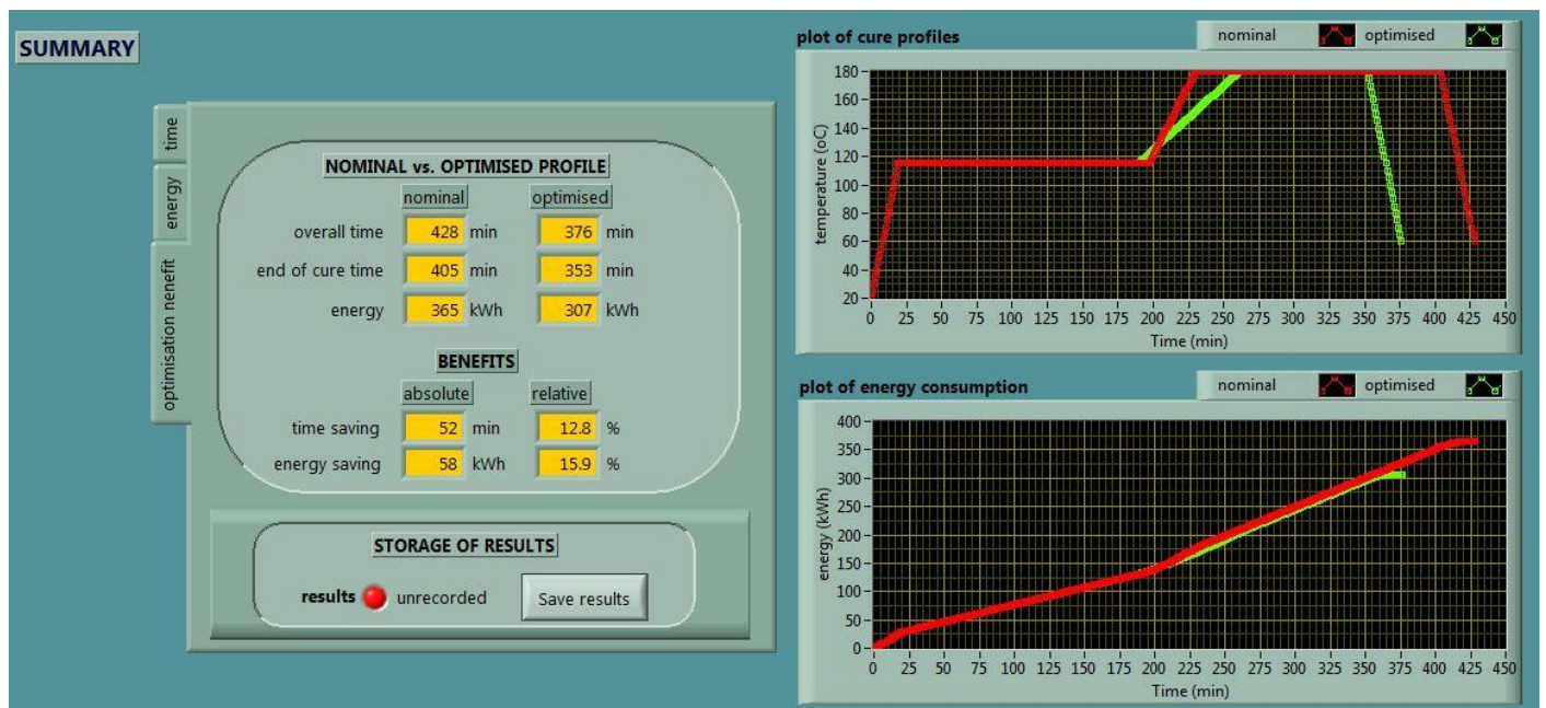
Figure 14: Summary tab for the operation of stage E in the cure profile optimisation module on the processing of large stiffened panels
