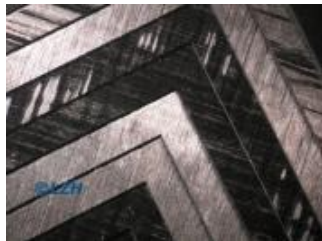
Laser ablated material (by LZH)
