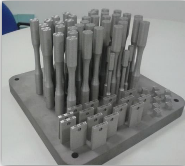
Figure 3. General view of the control samples manufactured with optimised parameters
