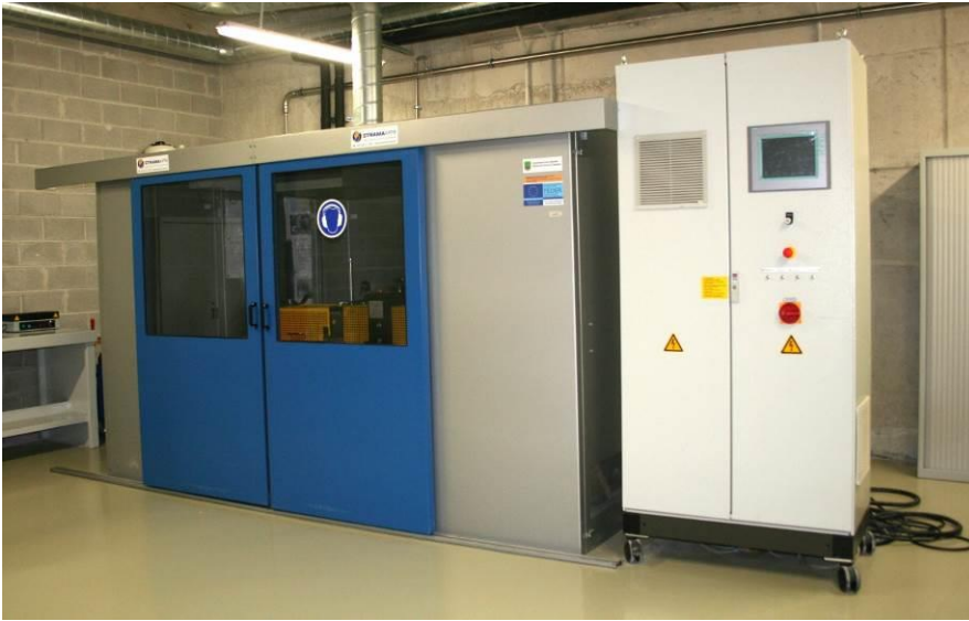
Figure 1 FZG gear test rig at IK4-TEKNIKER facilities (left) and detail of the gear test box (right)
