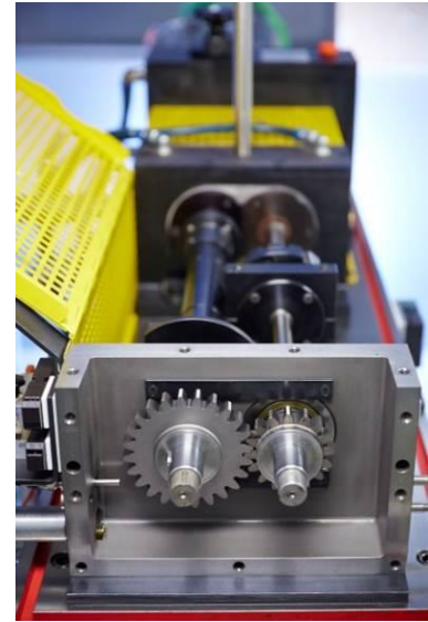
Figure 1 FZG gear test rig at IK4-TEKNIKER facilities (left) and detail of the gear test box (right)
