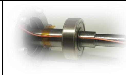
Figure 3.1.4 (a) Instrumentation of an induction machine rotor with 17 FBGs; (b) Fibre routing
