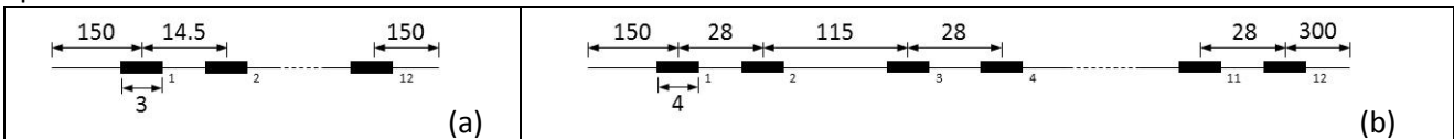
Figure 2.4 (a) FBG sensors to be circumferentially mapped onto the PM motor stator; (b) sensors to be installed along end-windings of the PM motor stator; (unit: mm)
