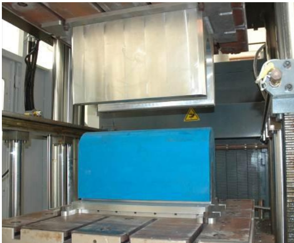
Figure 1: aluminium-rubber moulds used for the manufacturing of the skin of the sponson fairing
