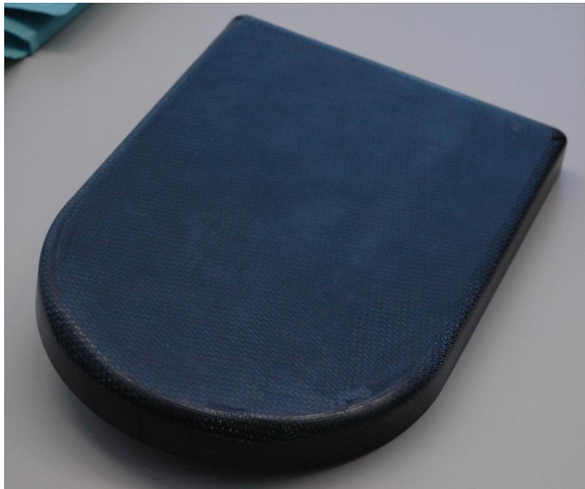
Figure 12: photo of the rib of the sponson fairing demonstrator.
