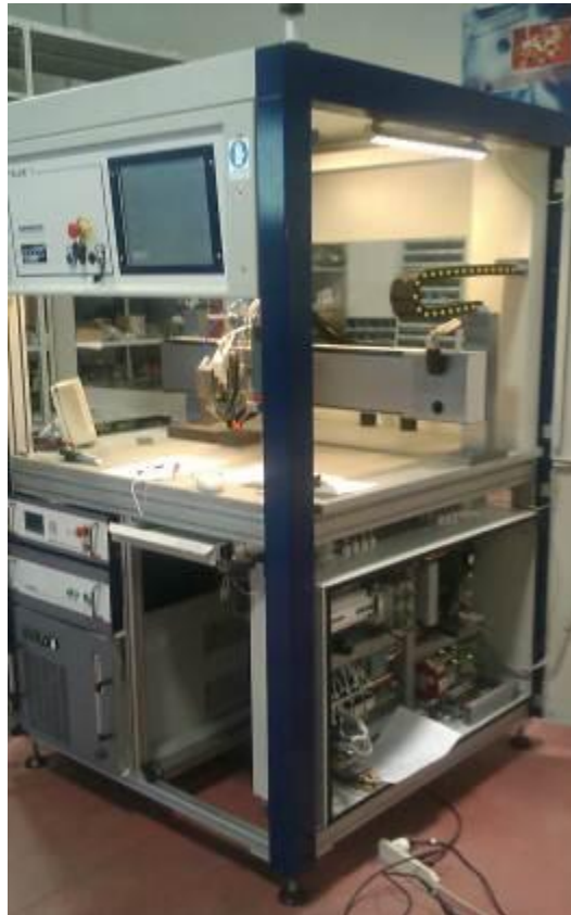
Figure 2: New induction welding machine for thermoplastic composites developed by CETMA and SINERGO, internal view.
