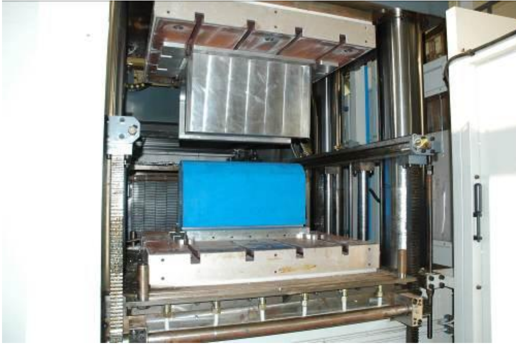
Figure 9: mould used to manufacture the skin of the sponson fairing.
