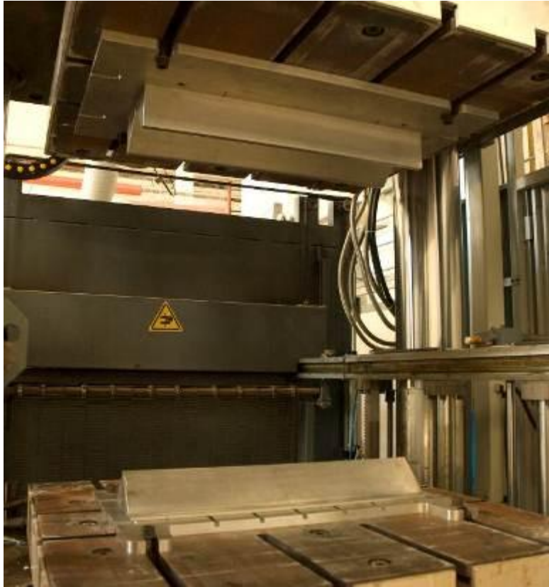
Figure 6: photo of the moulds used for the stringers manufacturing.
