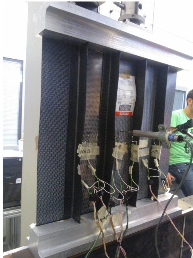
Figure 18: photo of the compression test on the upper panel.
