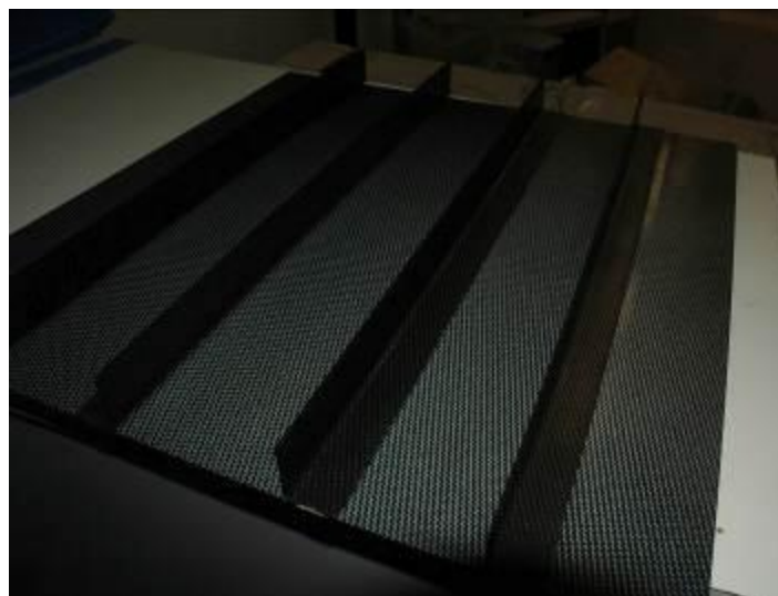
Figure 7: photo of the stiffened panel.
