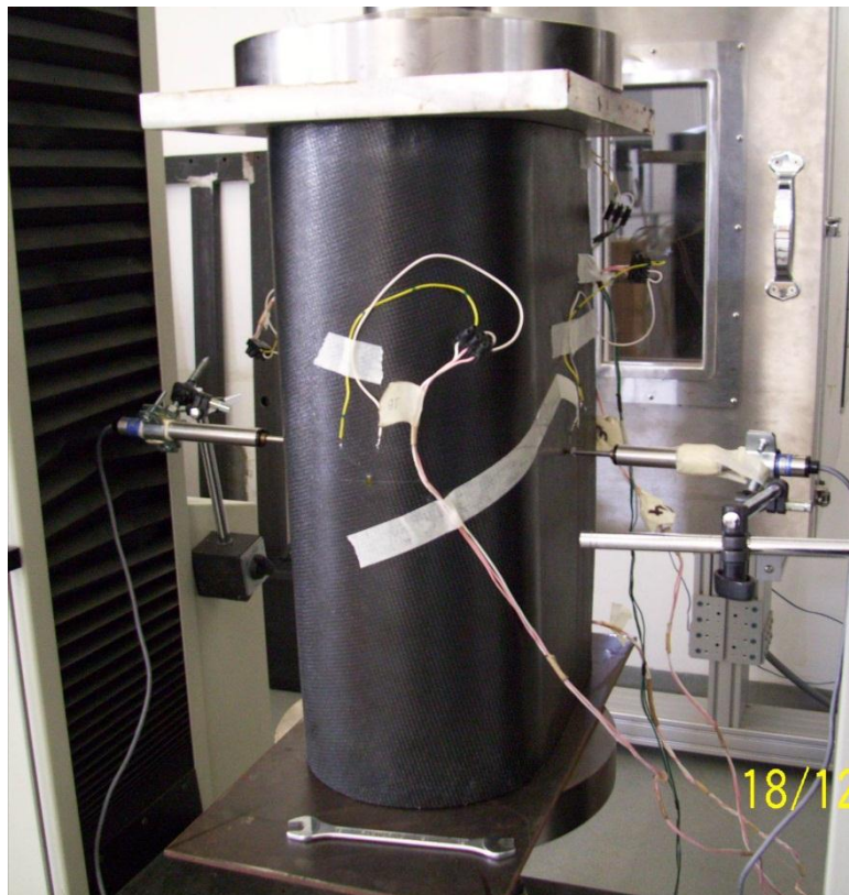
Figure 20: photo of the compression test on the sponson fairing.
