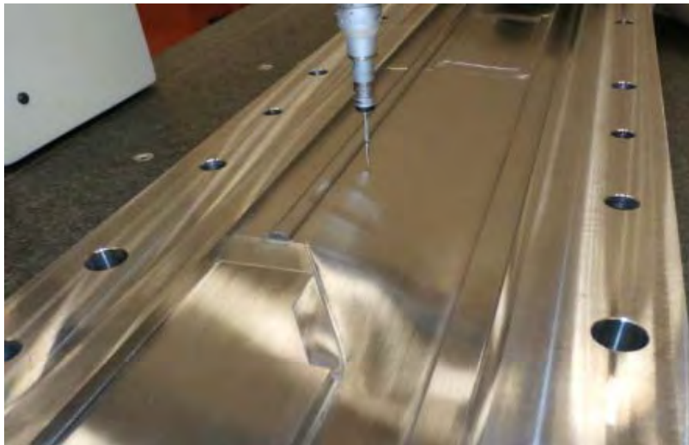
Figure 6 Dimensional control of the tools
