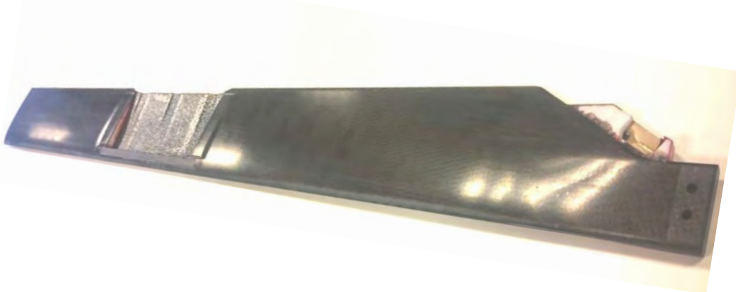
Figure 8 Rotorcraft model blade. First validation article produced
