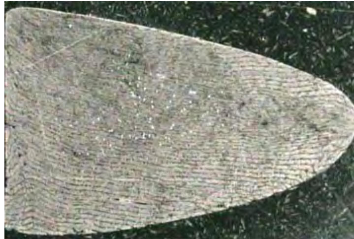
Figure 9 Optical microscopy analysis of a D-spar cross section
