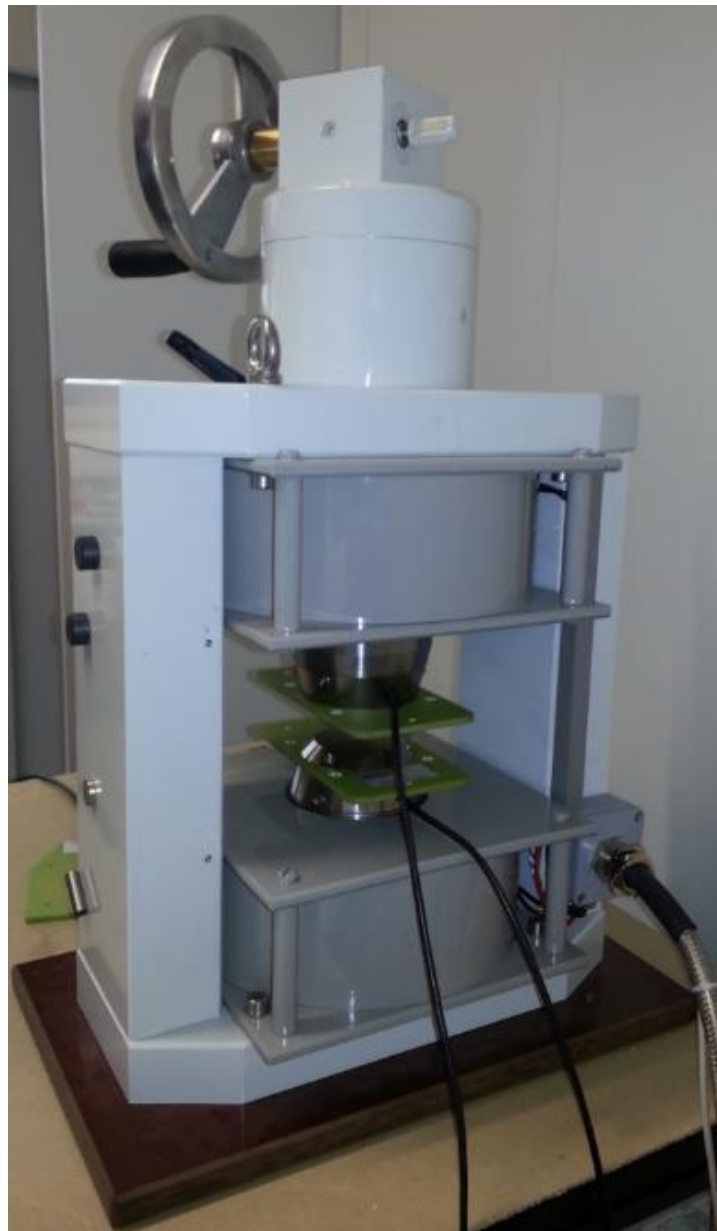
Fig 7. Electromagnet with integrated temperature and stress systems
