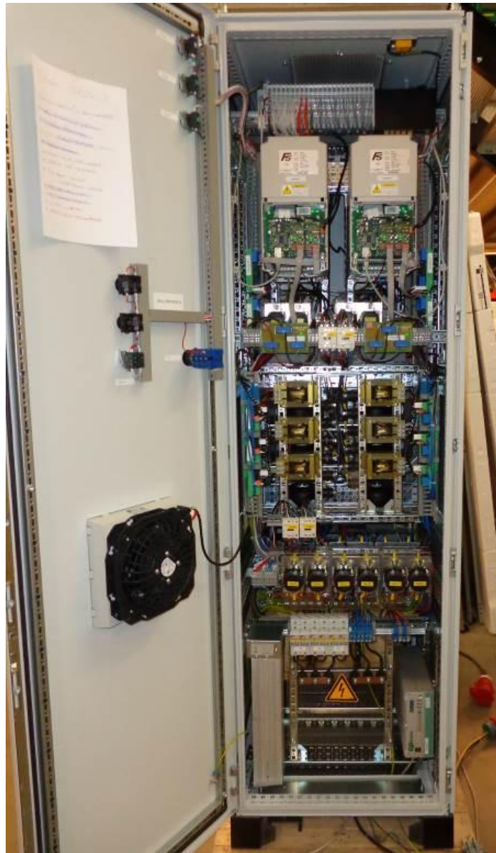
SPLS power flexible electrical load and source emulation power module.
