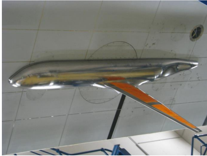
Figure 1: View on the wind tunnel ceiling mounted half model
