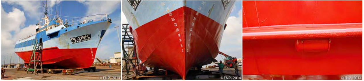
Figure 2. Vessel “Mar Português” painted with a new FOUL-X-SPEL silicone based non-leaching coating. Field trial test launched in September 2014. A drag friction prototype was fixed to the vessel (right).
