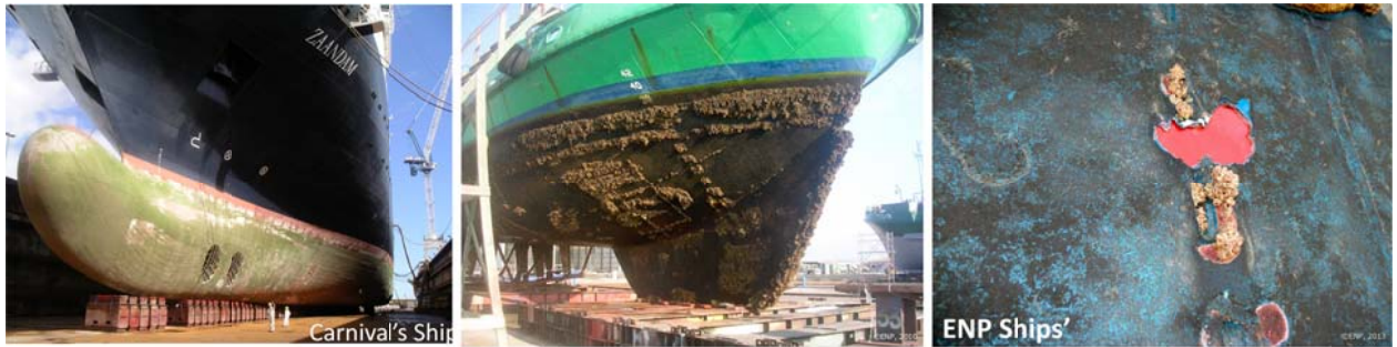
Figure 1. Biofouling on Ships' Hulls, which lead to organisms deposition and biocorrosion effects
