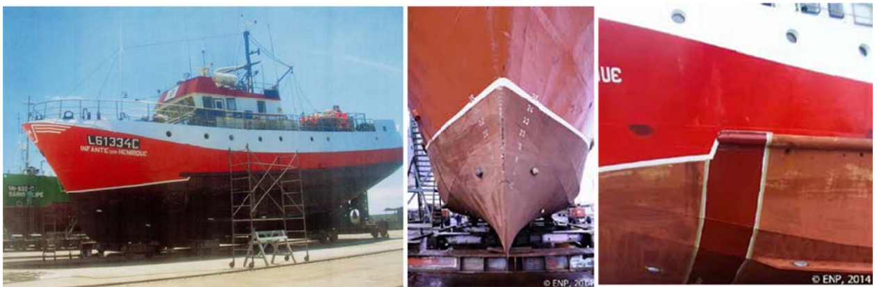
Figure 3. Vessel “Infante Dom Henrique” painted with a new FOUL-X-SPEL polyurethane based non-leaching coating. Field trial test launched in October 2014.
