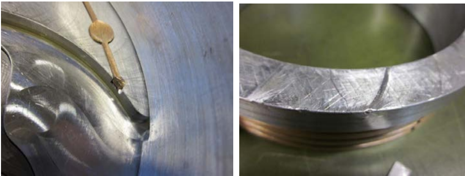
FIGURE 7 DAMAGED AREAS ON THE SIDE SEAL AND THE FOLLOWING ROTOR
