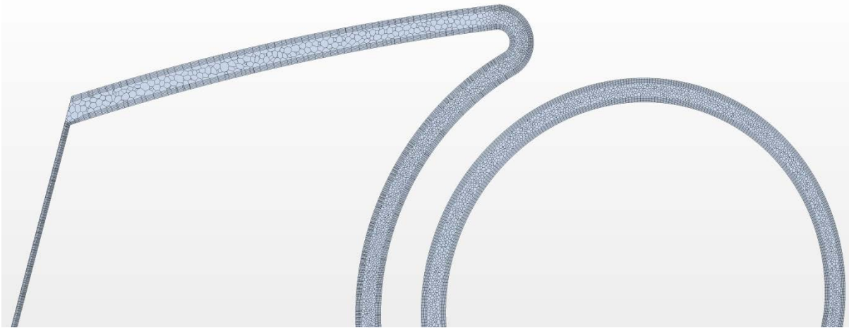
FIGURE 31 MESHING OF THE REGION AROUND THE SLIDER
