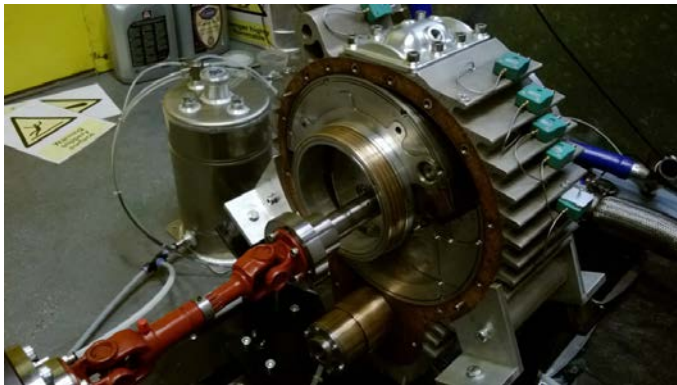
FIGURE 52 THE ENGINE ON THE TEST BENCH WITH ONE SIDE PLATE REMOVED SHOWING THE ROTOR
