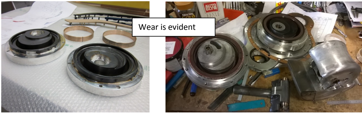
FIGURE 9 THE FRICTION MAINLY OCCURS ON ONE SIDE OF THE SIDE PLATE (TWO GENERAL VIEWS OF THE DISASSEMBLED ENGINE WITH WEAR EVIDENT ON THE LEFT-MOST OF THE TWO SIDE PLATES).
