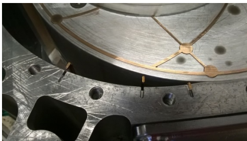
FIGURE 3 SEALS ON THE ENGINE BLOCK. ((C) ALSO SHOWS THE SEALING NETWORK ON THE SIDE OF THE ROTOR.)
