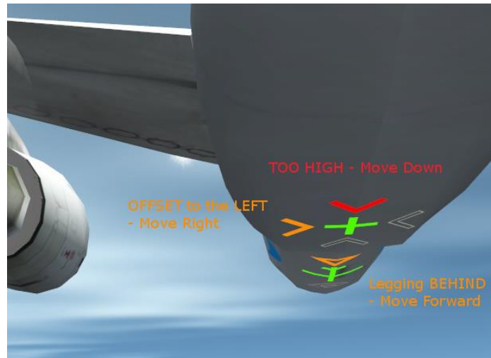
Figure 9: View from the cruiser cockpit of the safety indicators on the tanker aircraft
