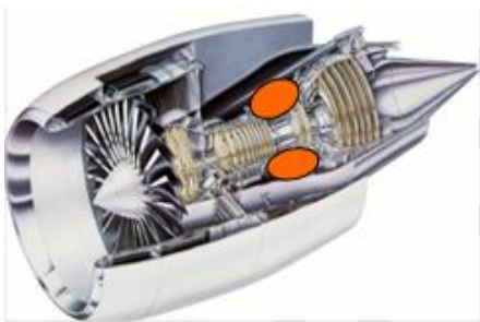
Figure 2.5.1: Space allocated for the combustor
