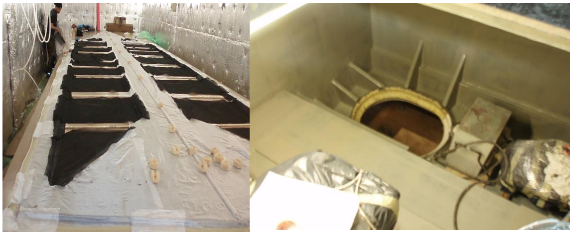
Illustration: Superstructure sides (left) and detail lamination for installation of pod propulsion.
