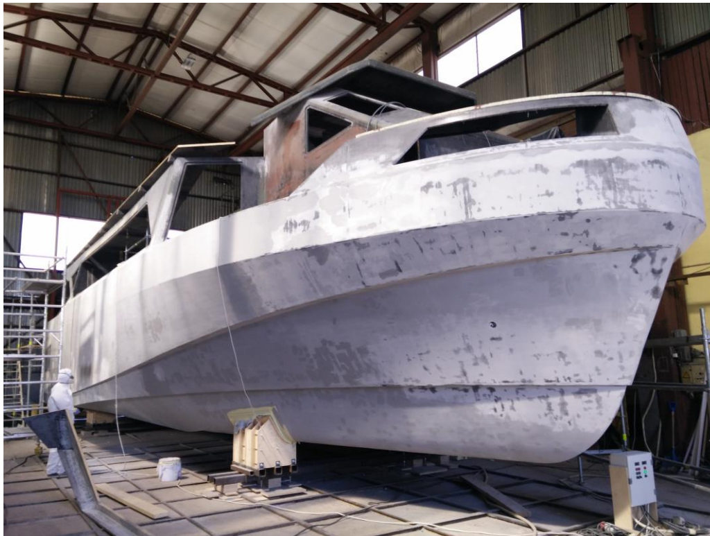
Illustration: From fairing and priming of hull, ready for paint.
