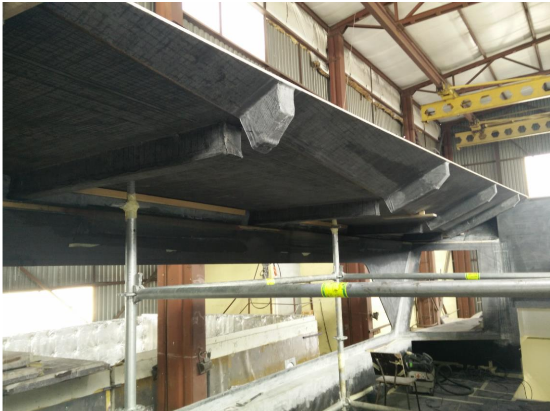
Illustration: A part of the superstructure roof section for the BB GREEN test vessel going in.
