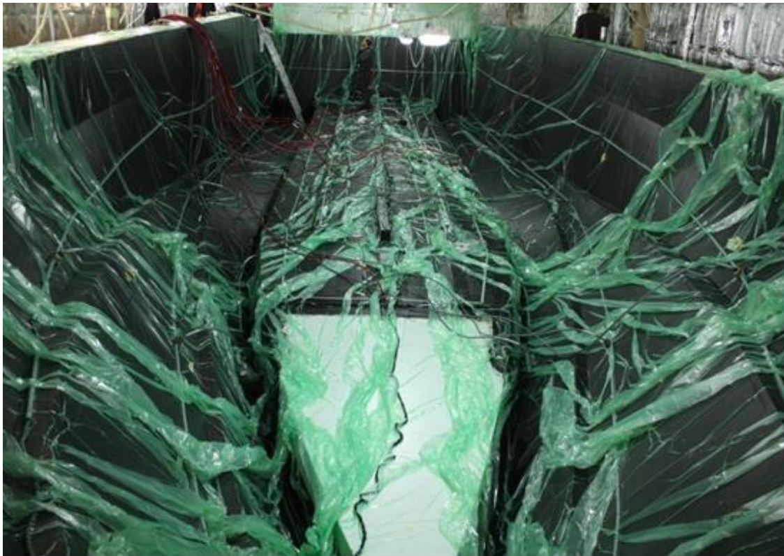
Illustration: 265 minutes after start up, infusion of hull completed.
