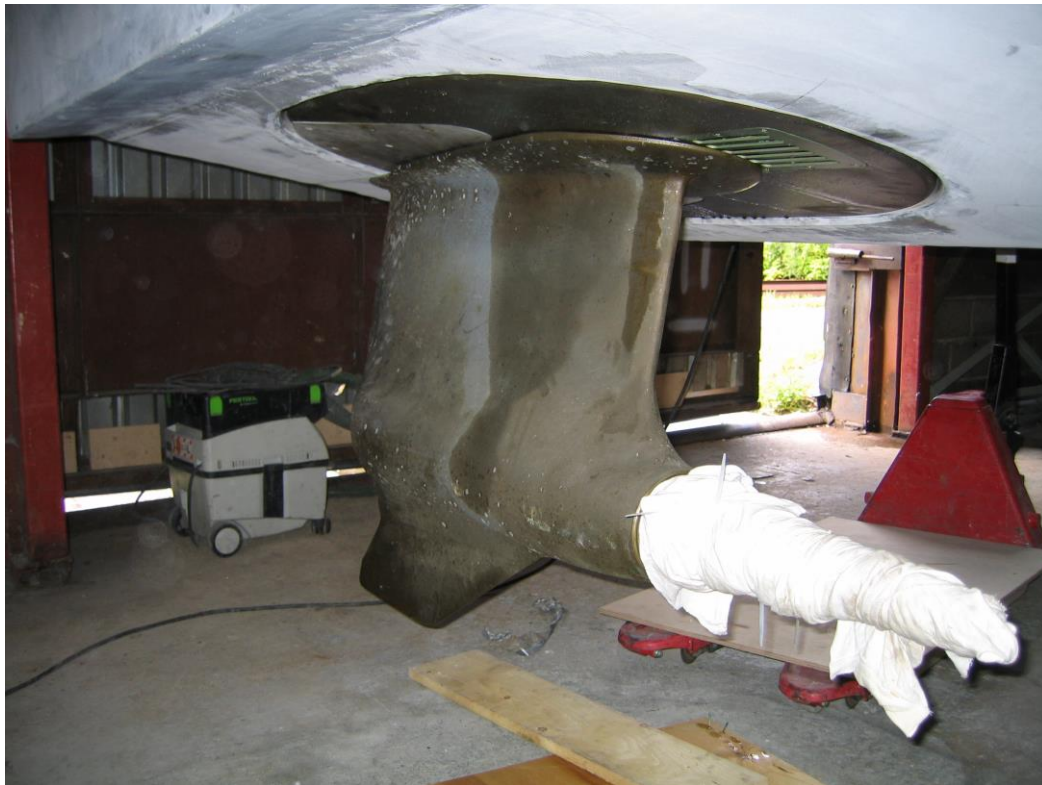
Illustration: From mounting of pod propulsion leg underneath the BB GREEN test vessel; the part of shaft covered by white cloth is where the twin contra rotating propellers will sit.
