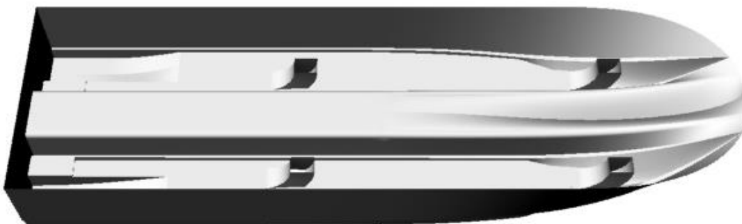
Illustration: BB GREEN ASV catamaran, showing with 4 lift fan air ducts.
