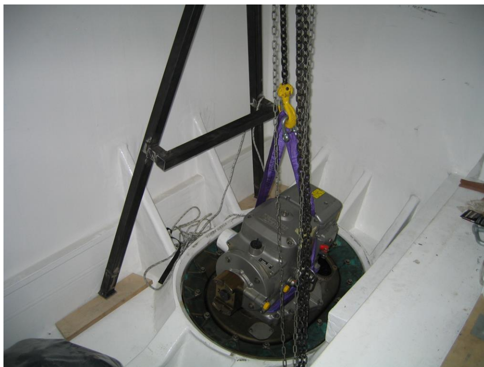
Illustration: From mounting of pod propulsion; showing on the inside of the BB GREEN test vessel hull.
