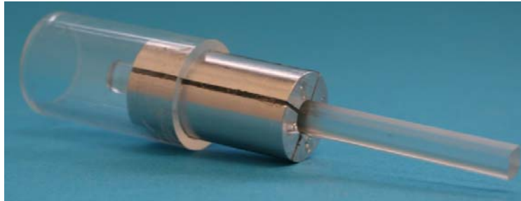
Figure 8 : Instrumented aluminium pin fin
