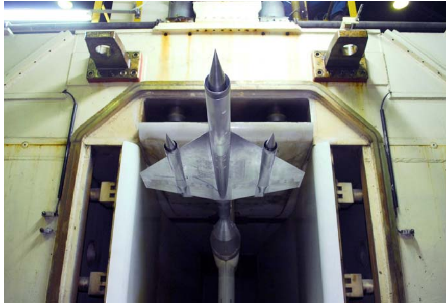
Figure 18: The transonic wind-tunnel-model with interior flow-path for the baseline
