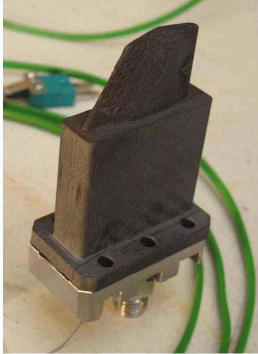
Figure 34 : post-test view of transpiration-cooled CMC generic strut
