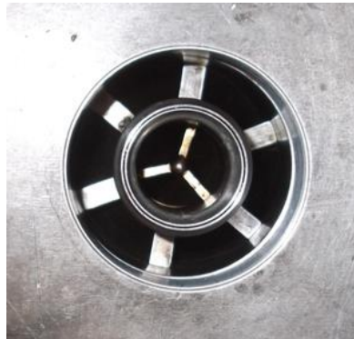
Figure 15: ONERA injector geometry: Injector outlet
