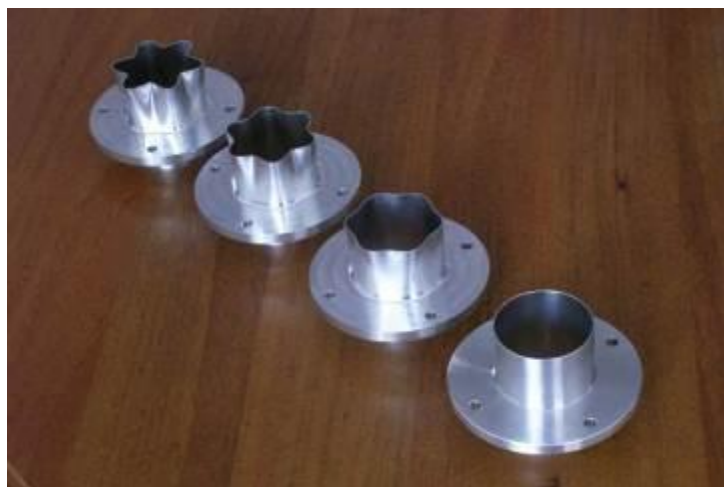
Figure 2. Corrugated nozzle family with equivalent area of the output cross section
