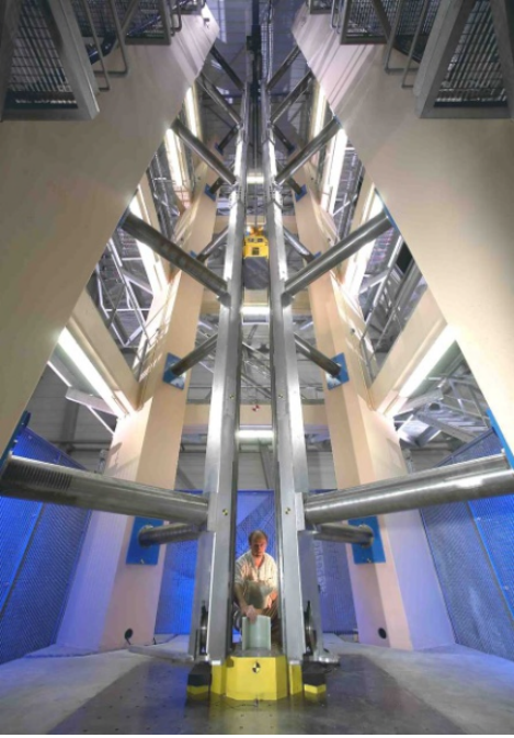
Figure 8: ONERA crash tower facility used for dynamic structural characterisation test.
