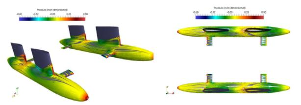
Fig. 7. Swath in fully appended configuration. Limiting streamlines colored with surface pressure.
