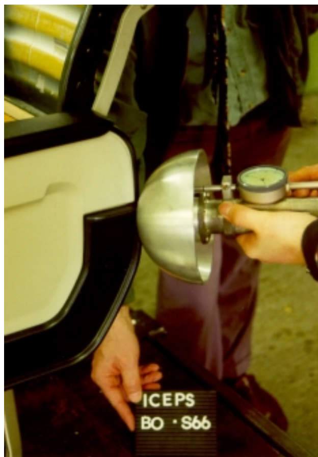
Figure 5.3-9 Spherical headform apparatus for measuring projections and edges
