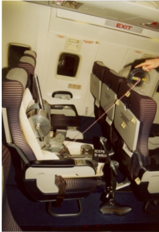
Figure 5.6-9 determination of the head impact area
