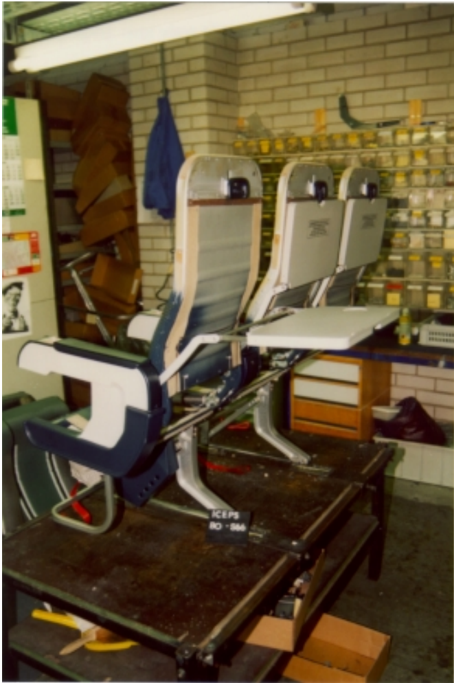
Figure 5.6-11 Passenger seat without padding, total view
