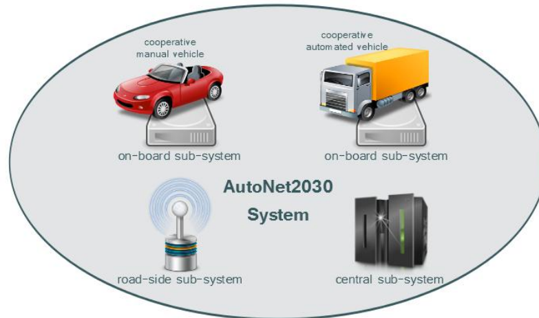
Figure 4 - AutoNet2030 system structure
