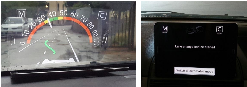
Figure 20 AutoNet2030 HUD (left) and secondary (right) realistic projections
