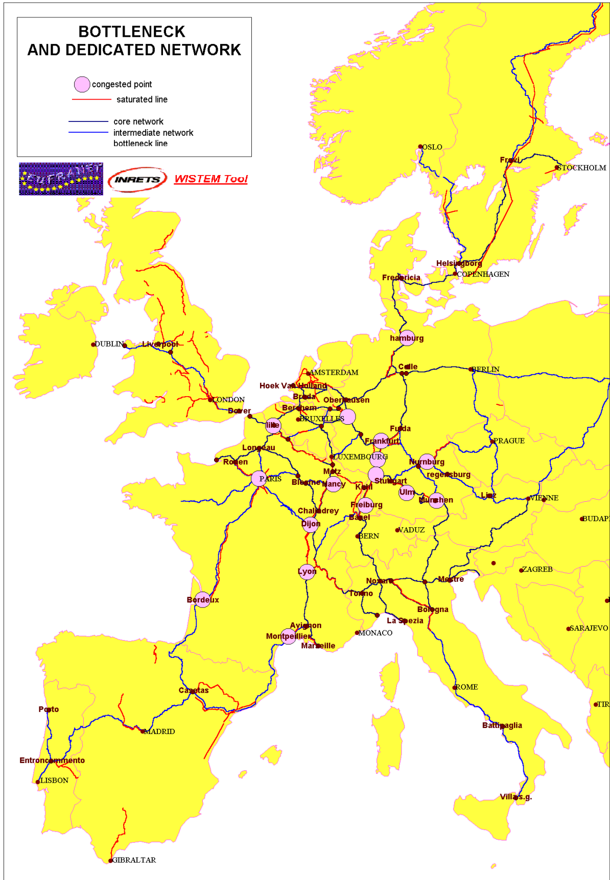
Figure 6.3. Map showing dedicated network with bottlenecks and black spots (source : SNCF, DB, EU)
