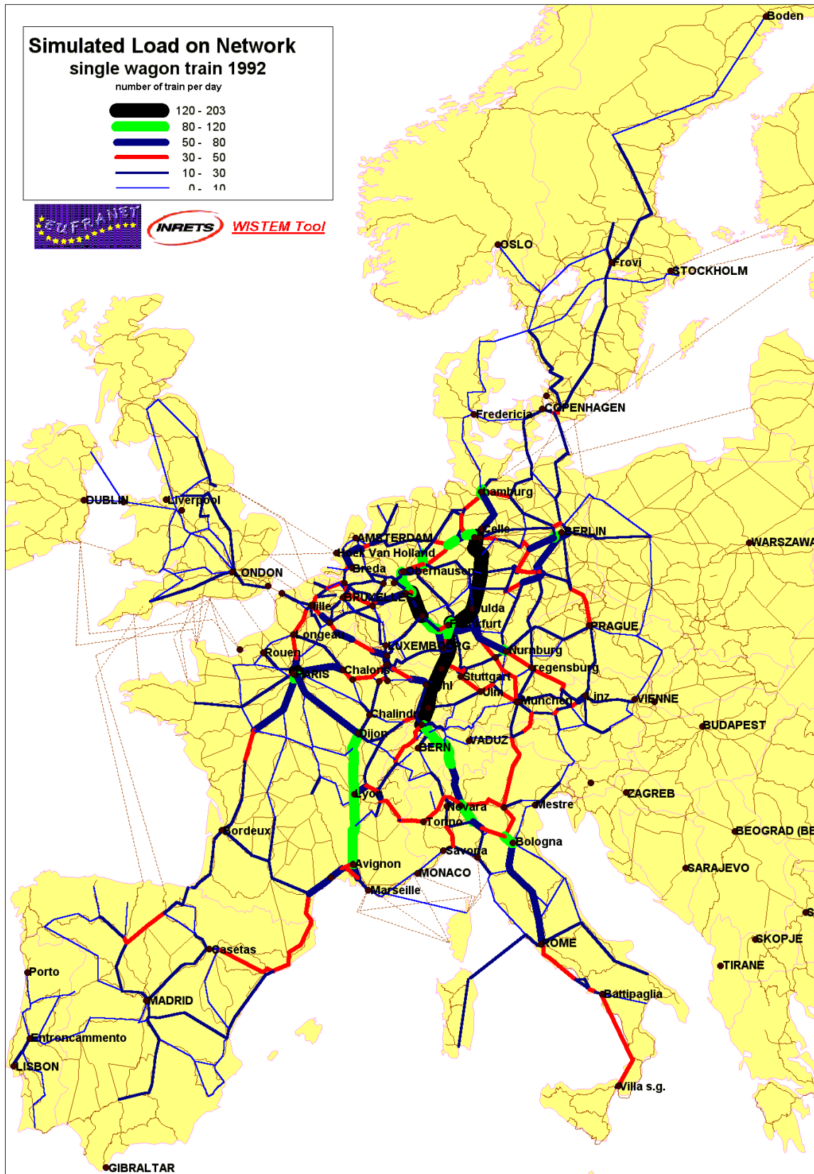
Figure 4.3. Simulated load on network in 1992 - single wagon trains (source of assignment data : IVE)
