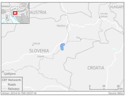
The Slovenian railway line "Celje-Pragersko" is located on the Baltic-Adriatic and Mediterranean Core Network Corridors. The line currently represents a bottleneck in passenger and freight transport due to insufficient load capacity and limited interoperability. The Action concerns construction works for upgrading of the "Poljčane-Slovenska Bistrica" double-track section with the main objective to increase the load capacity and improve the interoperability of the railway line.
