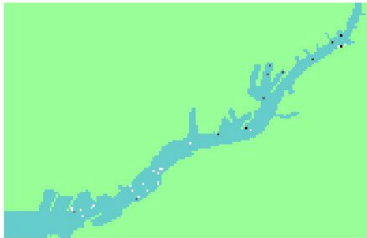
Fig. 41. Locations in Göteborg Harbour where the zinc concentration is likely to exceed 200 ppm using fuzzy set theory.
