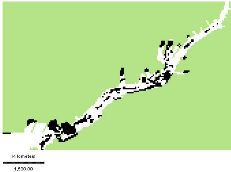
Fig. 44. Areas where there is a high probability of the sediment thickness layer exceeding 40 cm based on the ANN approach.
