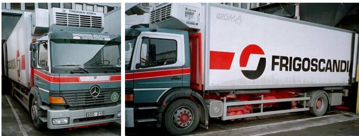
Figure 35: The refrigerated compartment is built on a Mercedes Benz Atego chassis
