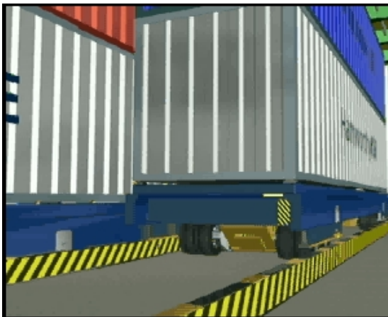
Figure 1-6. AGV carrying cassette with containers
