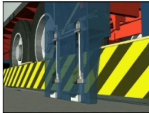
Figure 1-11. Automatic lashing of trailer horse
