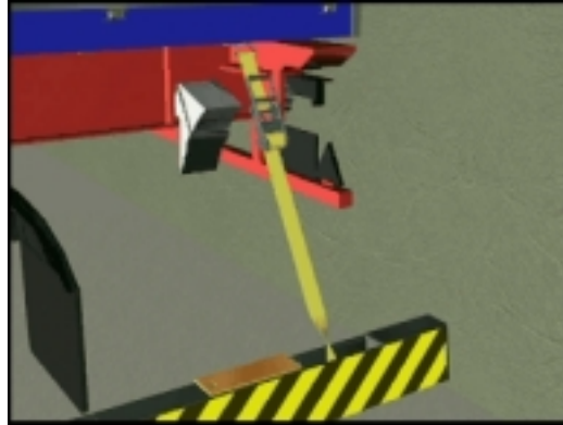
Figure 1-12. Manual lashing of trailers
