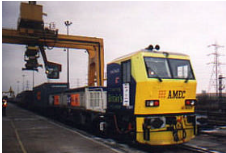
Figure 4.3/4: Loading TruckTrain at Freightliner's Barking Terminal by RMG
