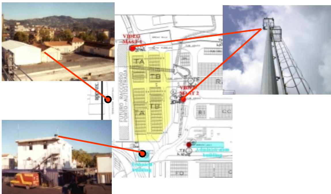
Figure 14: deployment of fixed transmitters on the test site during the preliminary tests
