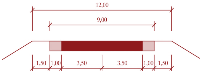
Recommended road cross-section. Road technical category - II
