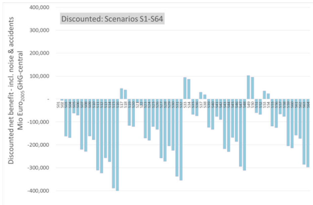
Figure 46: Discounted results of costs and benefits regarding internal and external costs for power plant and passenger cars of scenario S1- 64 compared to the reference scenario S1 (including greenhouse gases based on central value for GHG valuation, air pollutants, noise & accidents; accounting for costs of ETS certificates for the power plants) – [million €2005 ]
