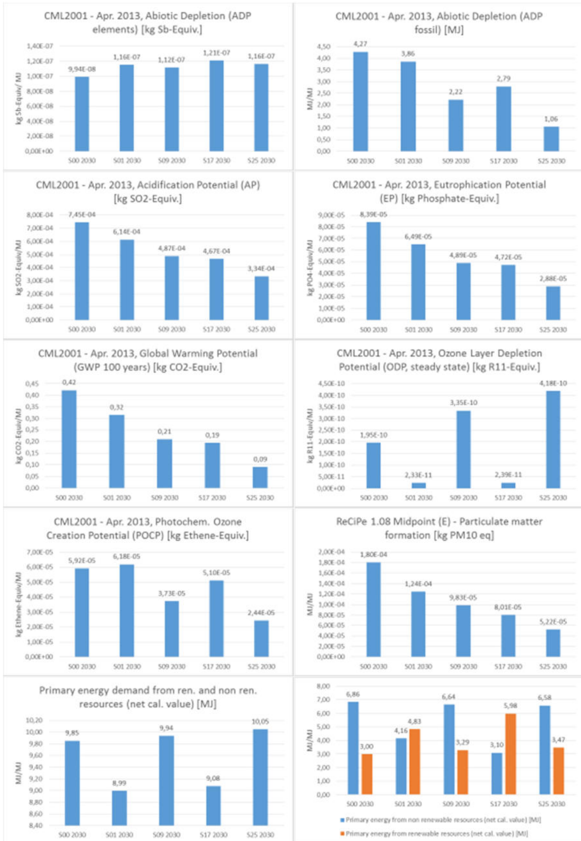
Figure 6: Environmental impacts of 1 kWh of electricity from the grid referring to different policy scenarios (S00, S01, S09, S17, and S25)
