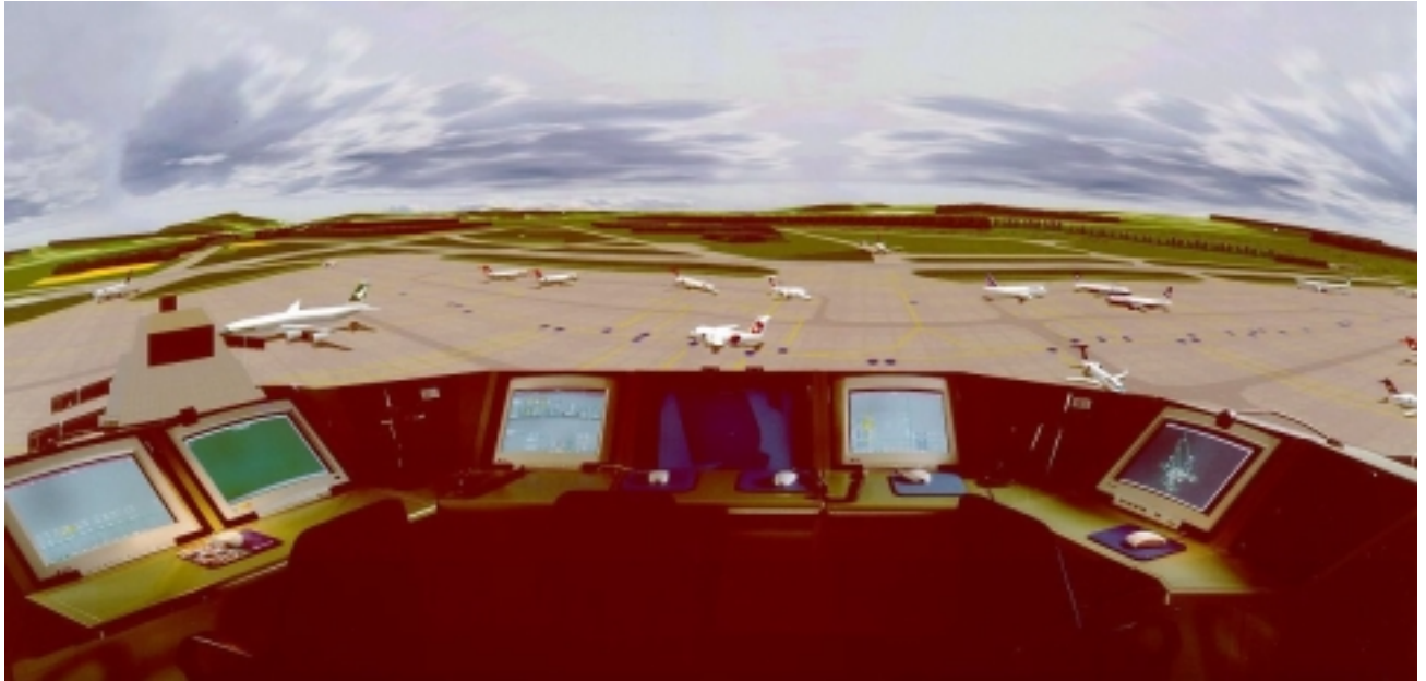
Figure 4, 300° Tower Simulator at DLR.
