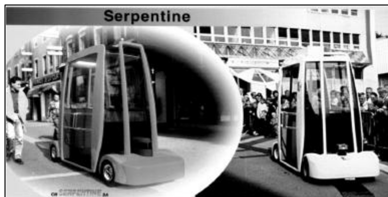
Figure 17 Serpentine shuttle in Lausanne, summer 1996, with induction band as power supply and guidance.
