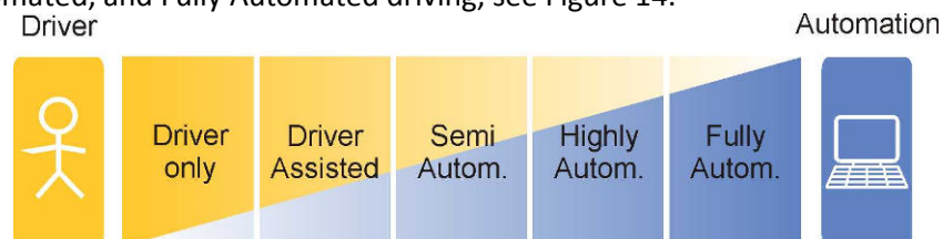
Figure 14: Possible levels of assistance and automation in a highly automated vehicle
