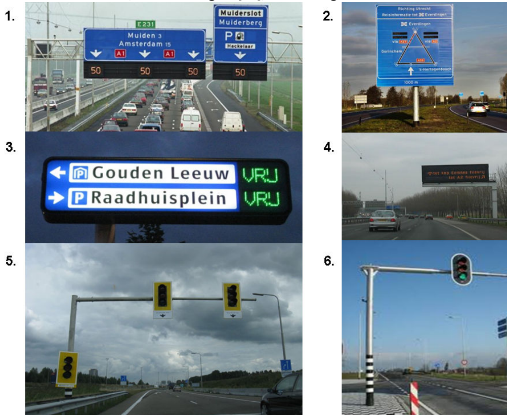
Figure 36: Current infrastructure communication technologies; dynamic road signs (1), GRIP (2), PRIS (3), DRIP (4), dosing system acceleration lane (5), traffic signs (6)
