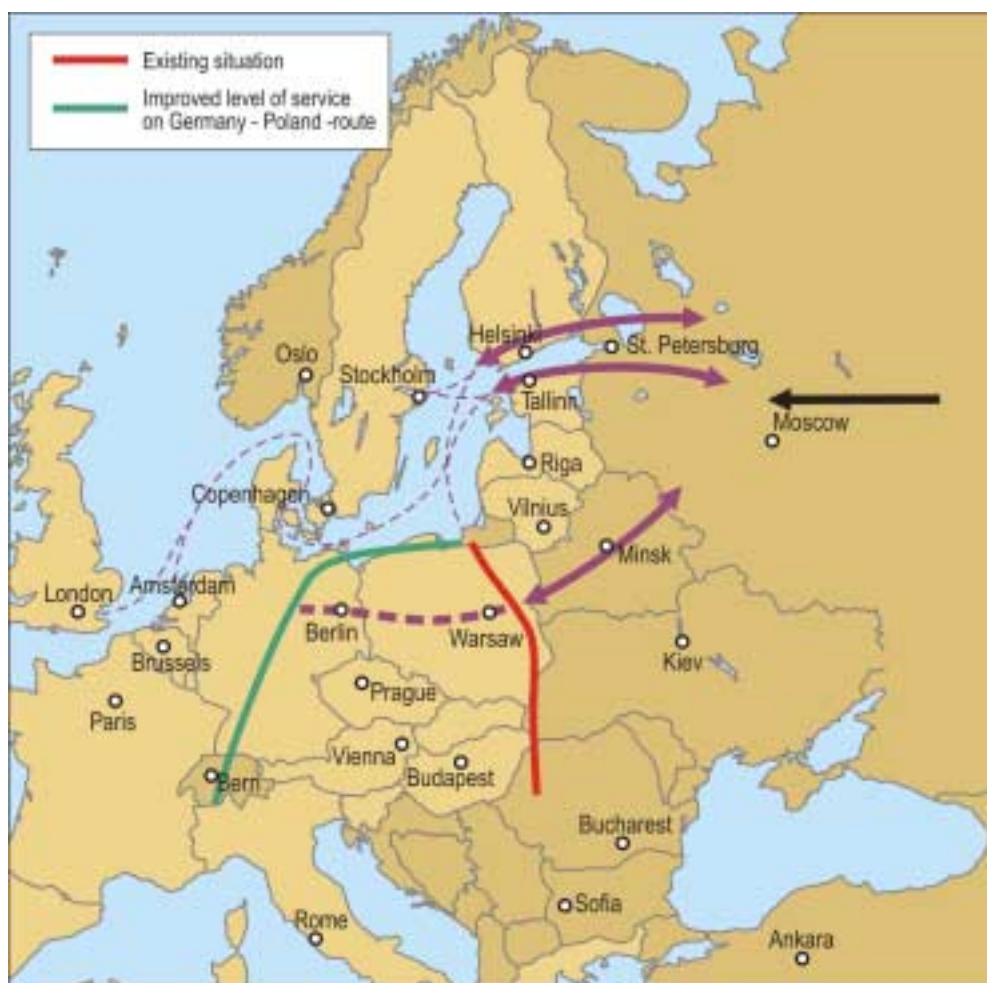
Figure 5.5. Transport routes of valuable products between Moscow and the EU: change of impact areas as a result of the improved level of service on the Germany–Poland–route. A road connection of motorway standard and direct block train connections from Moscow to Berlin were assumed to be constructed. Delays at border stations were assumed to be the same as the average in the EU area or 2–5 hours.
