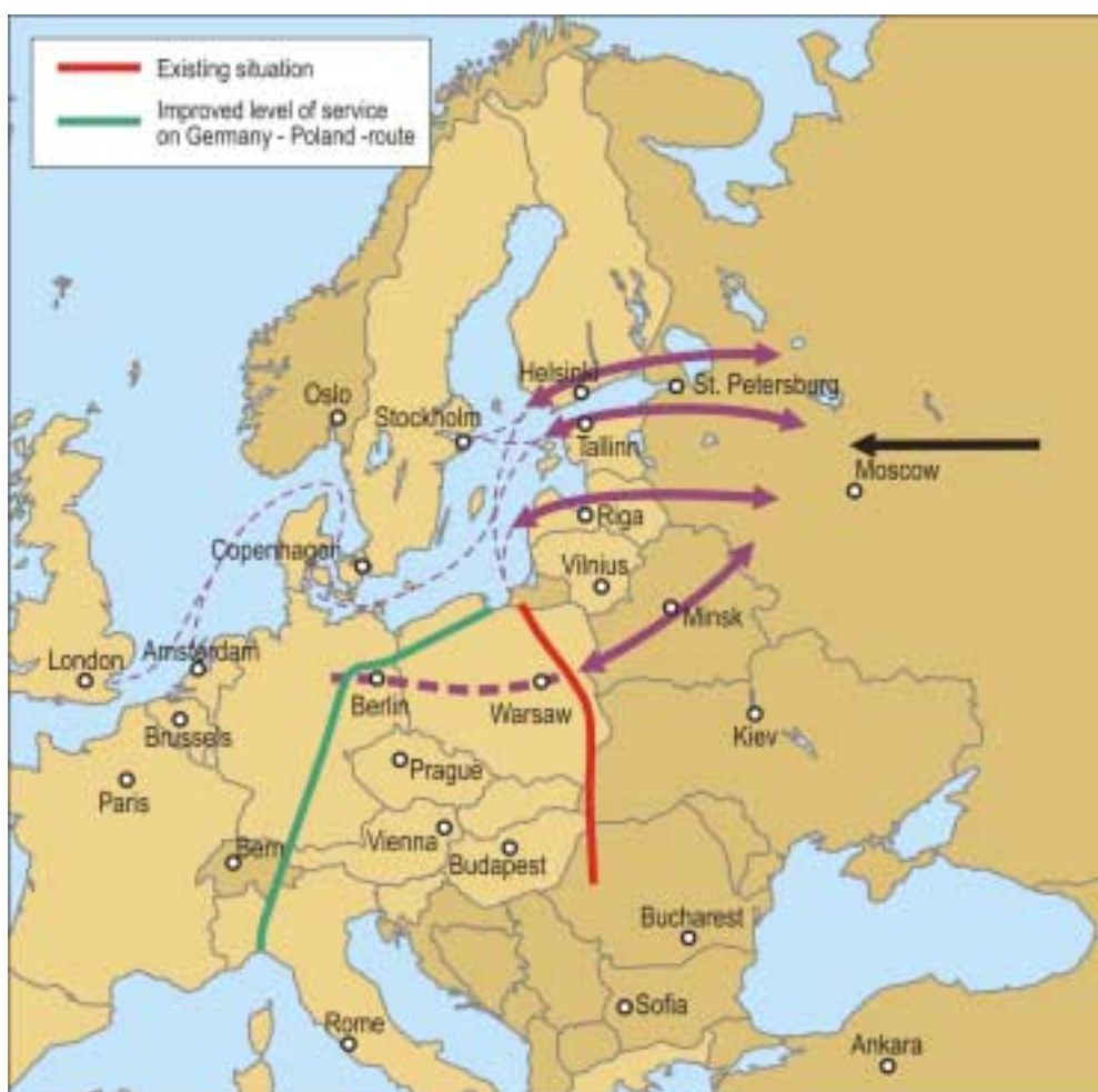
Figure 5.4. Transport routes of metal products between Moscow and the EU: change of impact areas as a result of the improved level of service on the Germany–Poland-route. A road connection of motorway standard and direct block train connections from Moscow to Berlin were assumed to be constructed. Delays at border stations were assumed to be the same as the average in the EU area or 2–5 hours.
