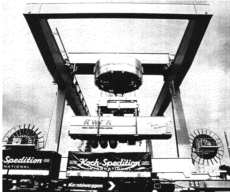
semi trailer prepared for lifting during the handling process in the grapppler arms of a spreader
