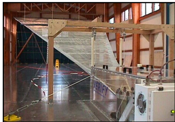
Fig. 3.21: Swiss VERIFY EMP simulation facility
