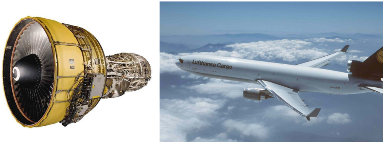
Fig. 46: Jet aircraft engine CF6-80 (left) which powers the aircraft MD11 Turbine (right)
