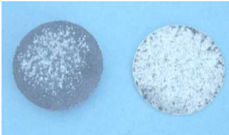
Fig. 24: Standard coating sample after thermal cycling
