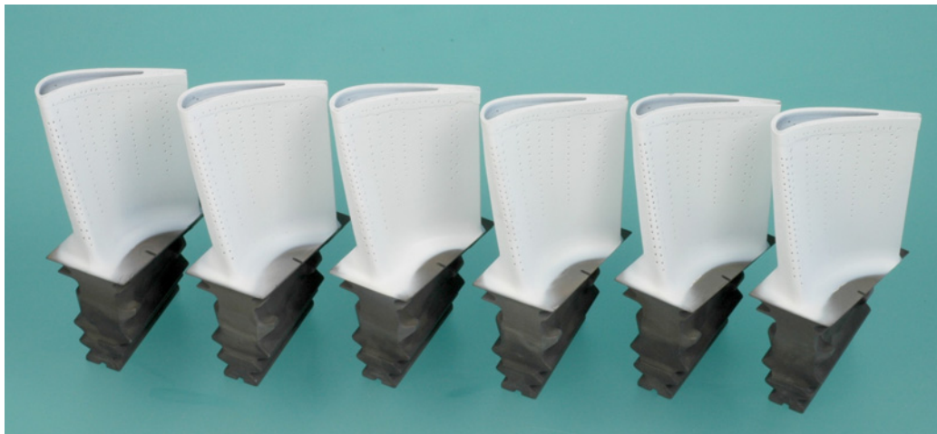
Fig. 40: Turbine blades (test samples / scrap) provided by LHT and coated by C-UK with the double EB-PVD TBC layer 7% YPSZ / 14% YSZ as coated for industrialisation process
