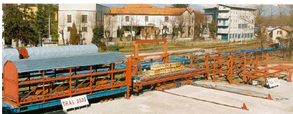
The TRAI 2000 system, a horizontal transshipment system, compatible with most terminals and permitting easy and economic automation
