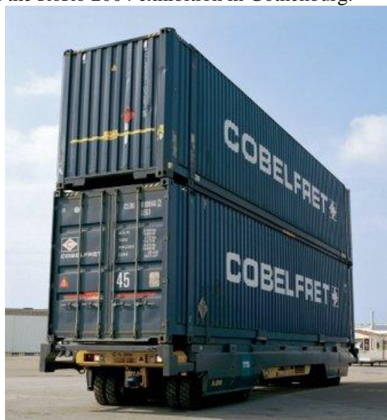
Two containers on a cassette transported by an AGV
