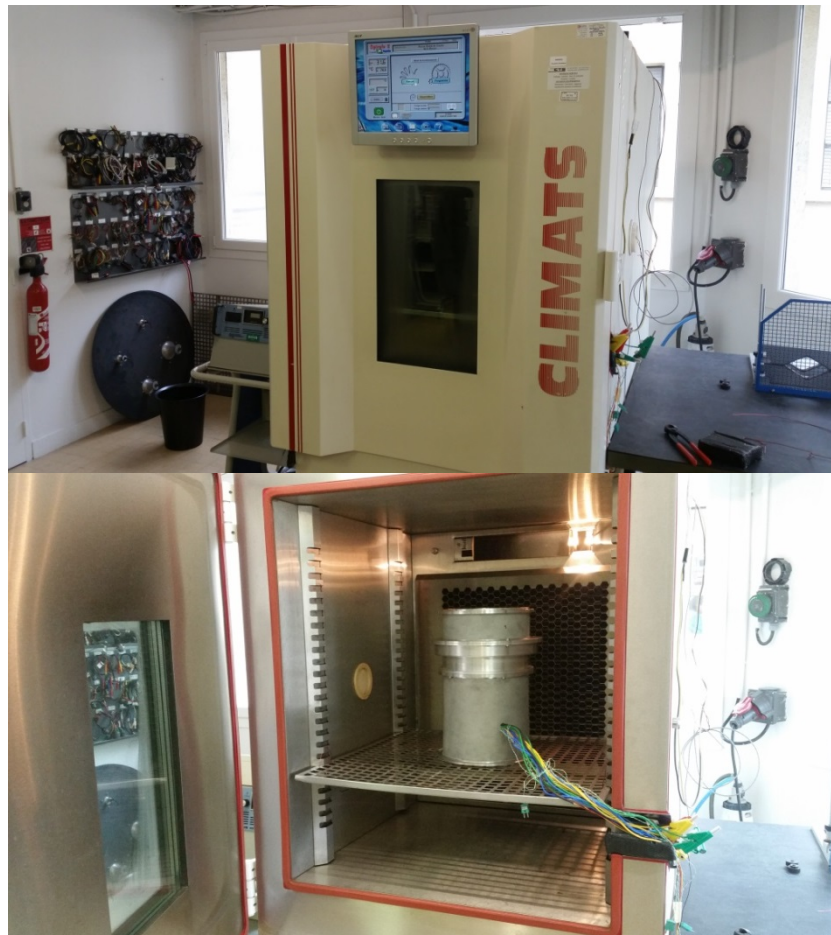
Figure 25 – LMB environmental test chamber to conduct the high temperatura tests required within EFFAN. In the picture below we can see the EFFAN fan prototype ready for testing
