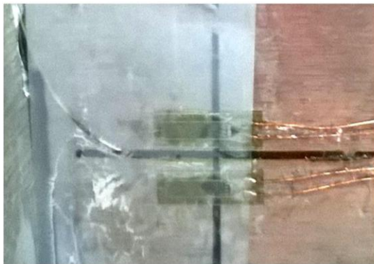
Figure 3: FBG 1 of fiber 1998A2 between SG 6 and SG 7.
